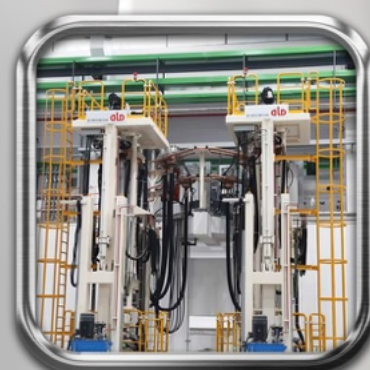
4 Sets of Two-Station Vacuum Arc Remelting Furnace with 10~15 ton
