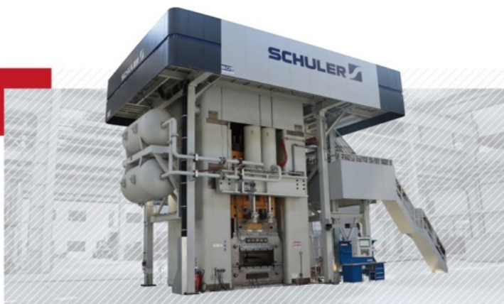
220MN Electric Screw Press: Designed and manufactured by German Schuler 20KN Railbound Robot Manipulator: Designed and manufactured by German Glama
