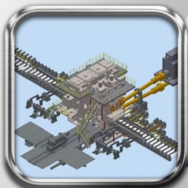
8000 Tons Reversible Hot Rolling Unit with 3000 mm width & four roller
